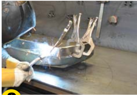
8 Once the inner wheelhouse is removed, weld the wheel tub filler in place.
