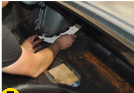
5 Tape the cutting line templates (included in the kit) in place and use spray paint to mark your cutting lines.
