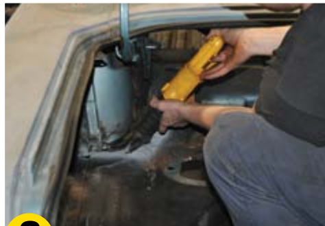
6 Following your painted cutting lines, use a Sawzall or other cutting tool to cut out your inner wheelhouse.
