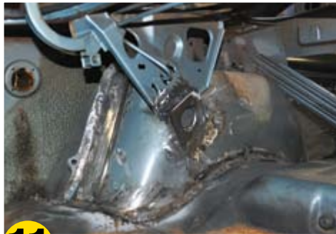
11 Be sure to weld the package tray brackets to your new widened wheel tubs and use the trunk hinge bracket in the kit to weld your trunk hinge brackets into place.
