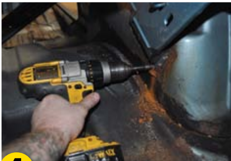
4 Drill out the spot welds holding the trunk hinge bracket to the inner wheelhouse.
