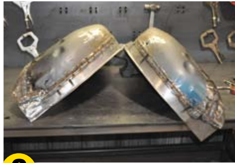
9 Here's what your widened wheel tubs should look like after you're finished welding.
