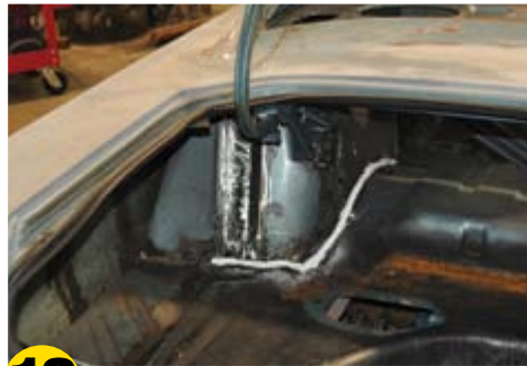
12 Use some seam sealer to fill any gaps just like the factory did. Now you're ready for some nice wide meats!
