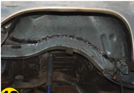
10 Weld your widened wheel tubs in place!
