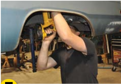
7 Use a Sawzall or other cutting tool to cut out your inner wheelhouse.
