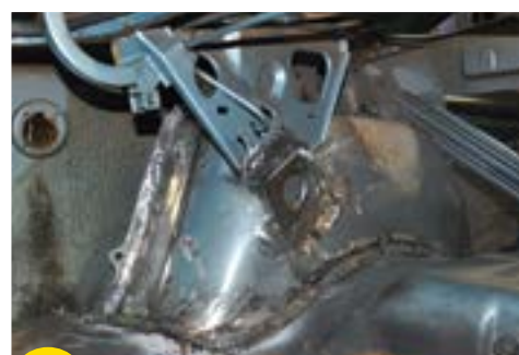
11 Be sure to weld the package tray brackets to your new widened wheel tubs and use the trunk hinge bracket in the kit to weld your trunk hinge brackets into place.
