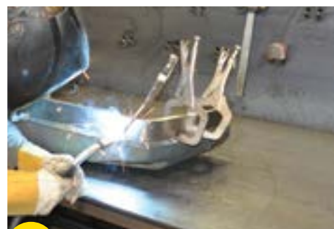
8 Once the inner wheelhouse is removed, weld the wheel tub filler in place.
