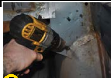
3 Drill out the spot welds holding the package tray bracket to the inner wheelhouse.
