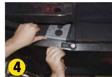
4 Carefully locate the new rear spring hanger mount.
