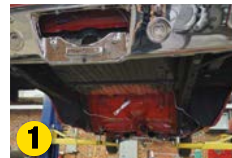
1 Disassemble the car, removing the rear axle, springs, mounts, and shocks. Also remove the fuel tank and filler tube.
