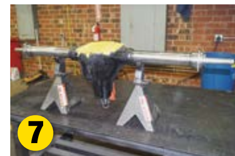
7 Prep your rear axle housing for the new relocated spring perches, mockup the rear-end and tires/wheels in the car, DO NOT MEASURE!
