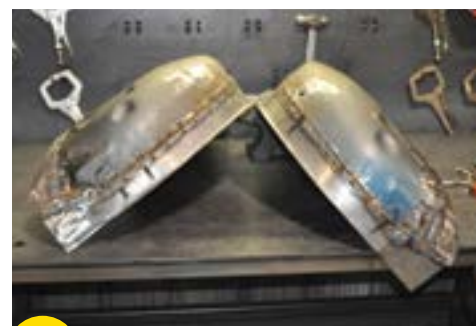
9 Here's what your widened wheel tubs should look like after you're finished welding.
