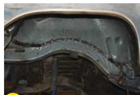
10 Weld your widened wheel tubs in place!
