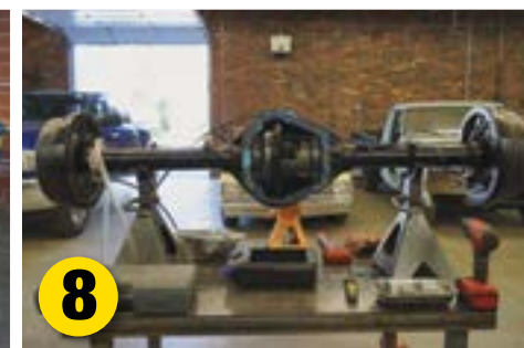
8 Double check after tack welding the perches in position, then weld them to the axle housing.
