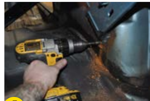
4 Drill out the spot welds holding the trunk hinge bracket to the inner wheelhouse.
