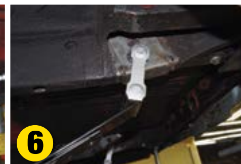
6 Fully weld the new rear spring hanger mounts (shown tacked in place).
