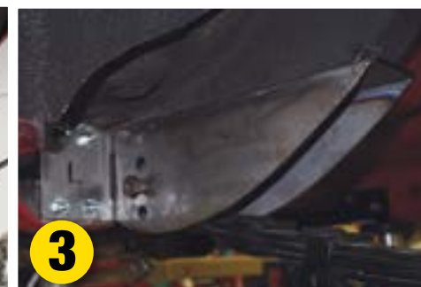
3 Carefully cut the frame rail, locate and tack weld. Mockup leaf springs in the front spring bucket. Confirm springs align with the rear frame rails.
