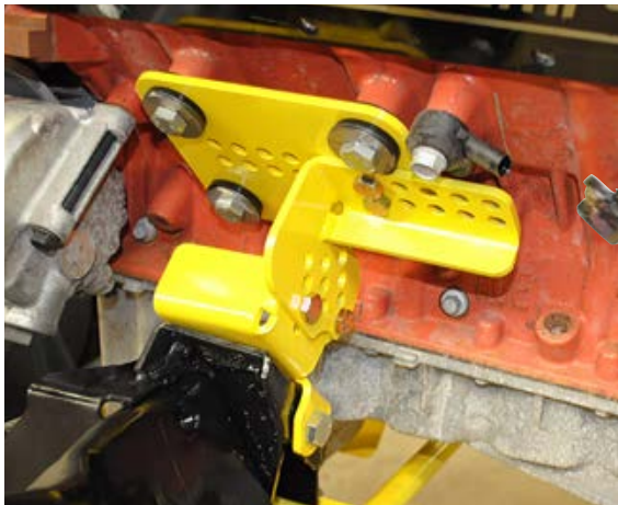
USCTAM2047 Gen 3 Hemi Swap Engine Mount kit to OEM K-Frame B, C, E Bodies
