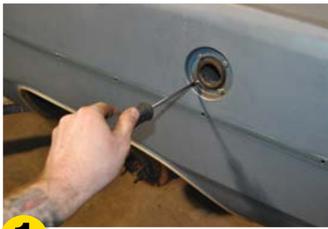
1 Disassemble the car, removing the back seat, decklid, fuel filler tube, etc.
