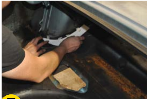
5 Tape the cutting line templates (included in the kit) in place and use spray paint to mark your cutting lines.
