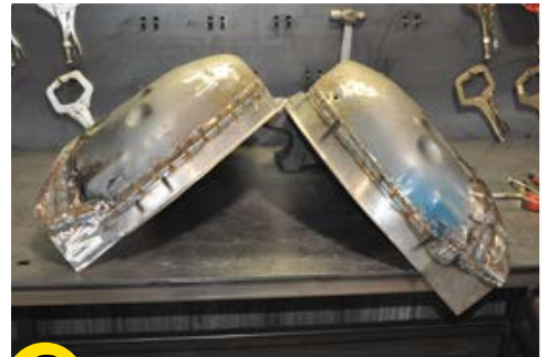
9 Here's what your widened wheel tubs should look like after you're finished welding.
