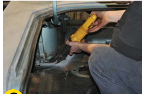
6 Following your painted cutting lines, use a Sawzall or other cutting tool to cut out your inner wheelhouse.
