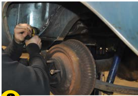
2 Using a spot weld cutting bit, drill out the spot welds holding the wheelhouse in the car.
