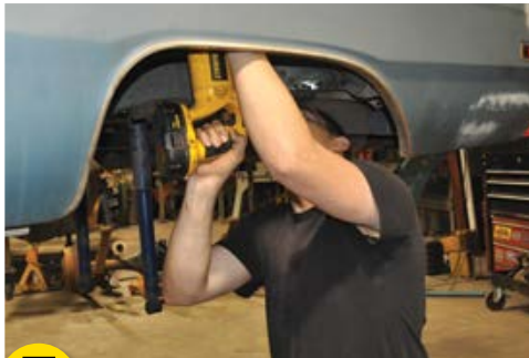
7 Use a Sawzall or other cutting tool to cut out your inner wheelhouse.
