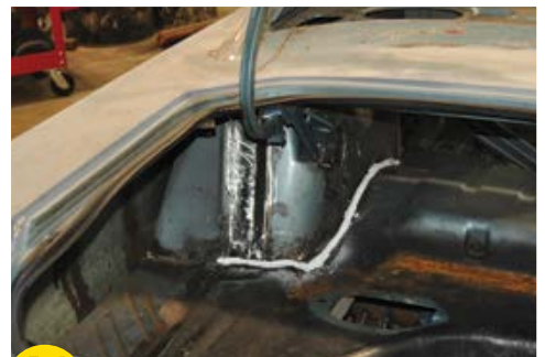
12 Use some seam sealer to fill any gaps just like the factory did. Now you're ready for some nice, wide meats!
