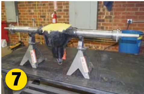
7 Prep your rear axle housing for the new relocated spring perches, mockup the rear-end and tires/wheels in the car, DO NOT MEASURE!
