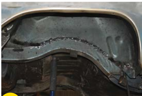
10 Weld your widened wheel tubs in place!
